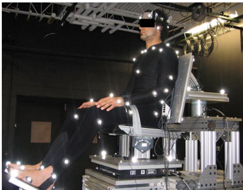
Figure 4.1 Experimental setup and marker locations on a participant sitting with the supported-back position
