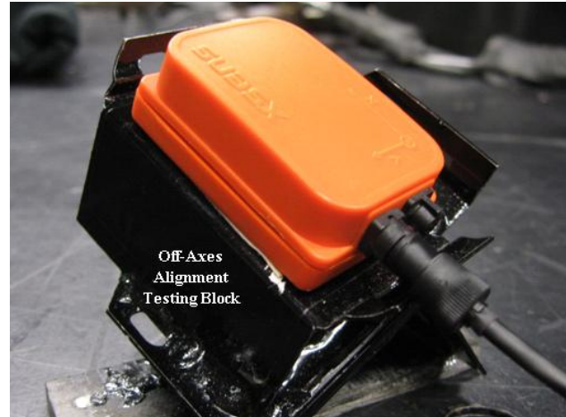
Figure 2.2 Testing block for dynamic vibration tests where all three sensor axes were rotated off-alignment from the global coordinate system. The testing block was rigidly attached to the motion shaker platform.
